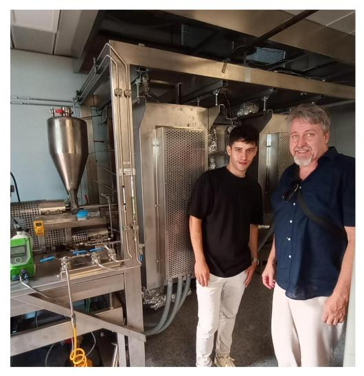
Xandre Costas (to the left) showed the fluidised bed gasifier and the subsequent catalytic tar reformer reactor.
