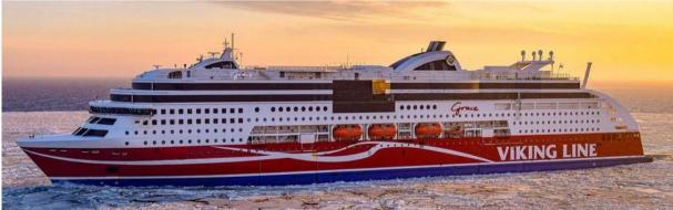
Viking Grace is 218 m long and has a capacity of 2 800 passengers. The gas engines have a capacity of 30 400 kW. The ferry was built in 2013.
