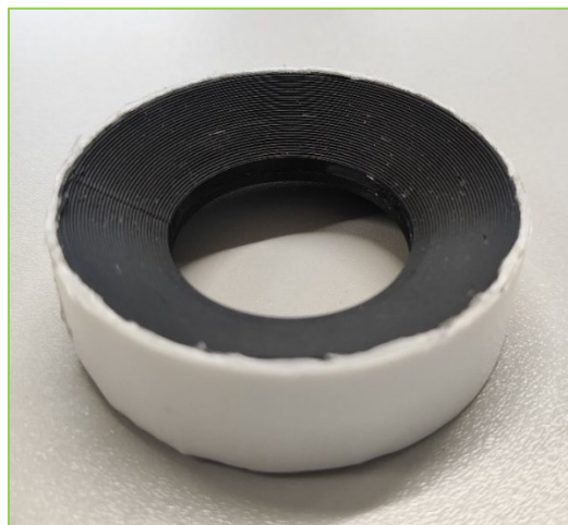
Figure 8 Example of a 3D-printed constriction, that is mounted in the CCC of the CFM.
