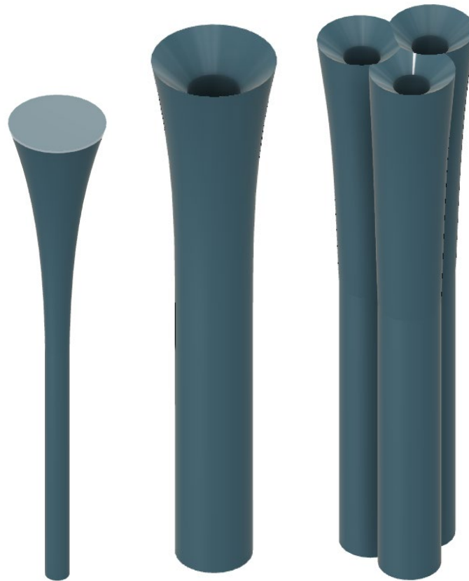
Figure 9: Comparison of the catalyst volume in the ADDmeth1, ADDmeth3.1 and ADDmeth3.2 designs
