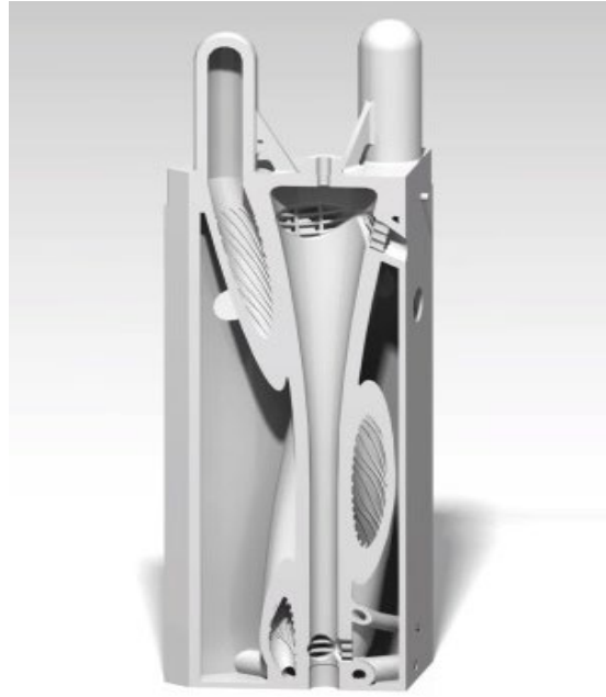
Figure 2: Cross-sectional front view of the conical reaction channel of the ADDmeth1 reactor
